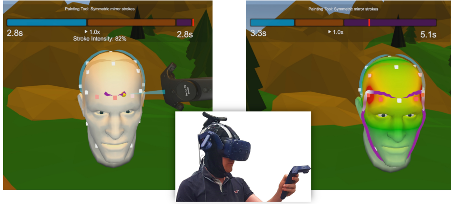
Fig. 1. The final version of VRTactileDraw in action. Users wear an HTC Vive Pro VR headset and a tactile display [26] (center). A user draws symmetric strokes on the 3D model head in VR (left) and then replays the resulting pattern (right). During drawing, the user can feel the resulting tactile actuation.
