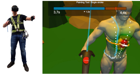
Fig. 13. VRTactileDraw driving the MultiWave prototype vest [41]: A wearable vibrotactile vest containing 76 actuators (left) and the user's view inside an HTC Vive (right). The user is replaying a TP and simultaneously feels vibrations as indicated by the heatmap.
