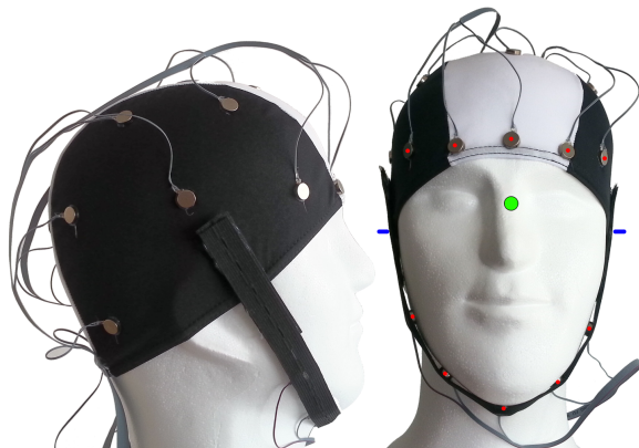
Figure 12. Second, refined HapticHead prototype, side and front view. Notice actuators located on the outside, the flexible chinstrap, and five instead of three actuators on each, the forehead and chinstrap. Positions of the 10 forehead and chin actuators forming a “ring” around the face are marked in red.
